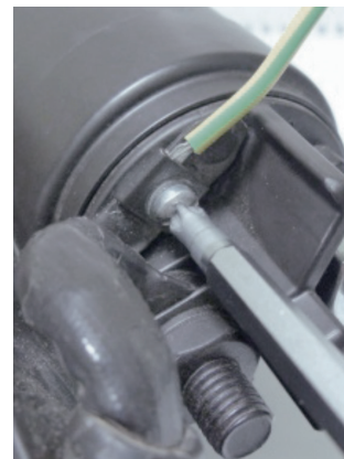
Figure 3: Cable attached to clamp 50 of the solenoid
