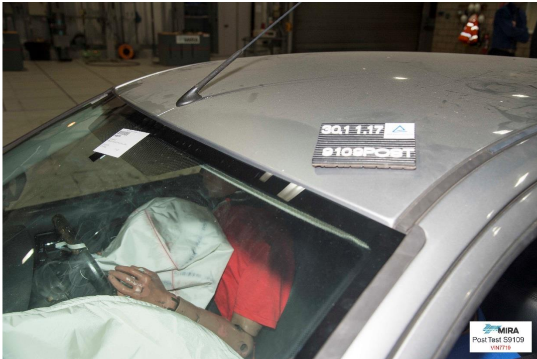
Photo 9 Close front view of header rail / windscreen top edge – Post-Test
